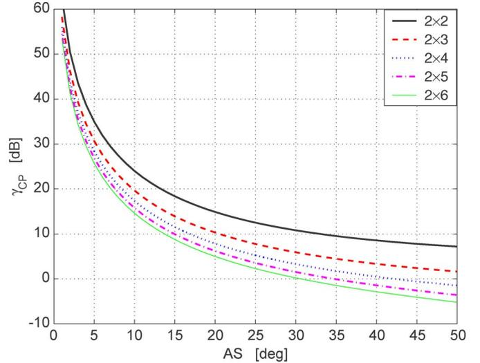
Fig. 5. Crossing-points for a MIMO  $(N_r, 2)$  system as a function of the AS and number of receive antennas  $(N_r)$ . Single-sided correlated channel with single cluster and mean angle of departure at  $0^\circ$  (broadside direction).
