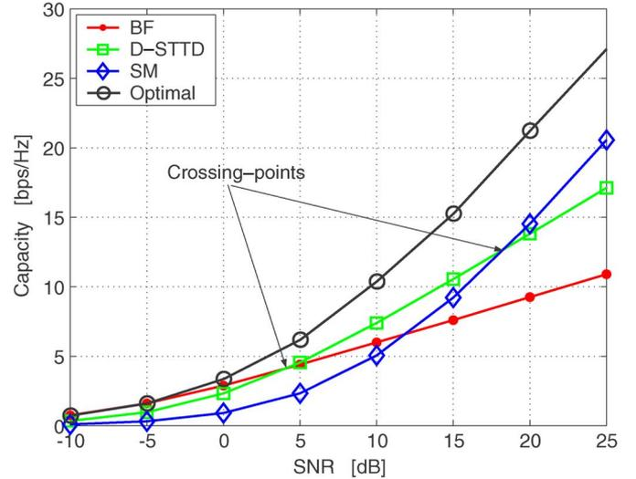
Fig. 3. Mean capacity for BF, D-STTD (with ZF), SM (with ZF), and optimal transmission in the IEEE 802.11n channel model F (NLOS).
