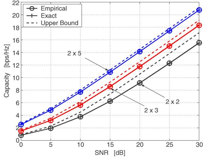
Fig. 2. Empirical, exact and upper bound to the ergodic capacity of  $(2 \times N_r)$  SM system with ZF receiver, in single-sided correlated channel model D (NLOS).
