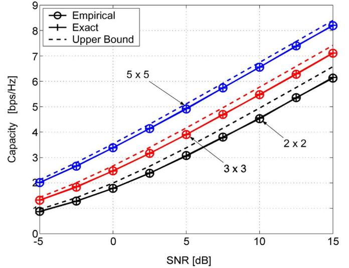
Fig. 1. Empirical, exact, and upper bound to the ergodic capacity of BF, in double-sided correlated channel model D (NLOS), with different antenna configurations ( $N_t \times N_r$ ).
