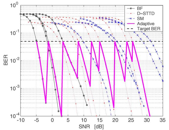
Fig. 6. BER of the adaptive MIMO transmission scheme versus fixed BF, D-STTD, and SM with different MCS, in channel scenario 4.
