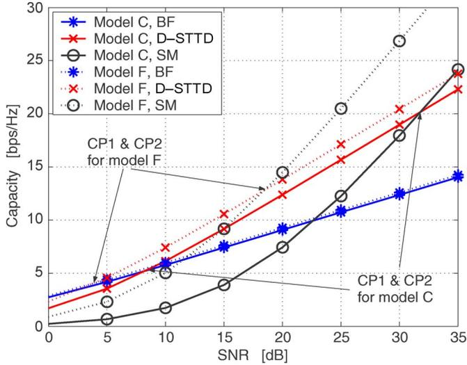
Fig. 4. Mean capacity for BF, D-STTD (with ZF), SM (with ZF) in the IEEE 802.11n channel models C and F (NLOS). CP1: crossing-point BF versus D-STTD; CP2: crossing-point D-STTD versus SM.
