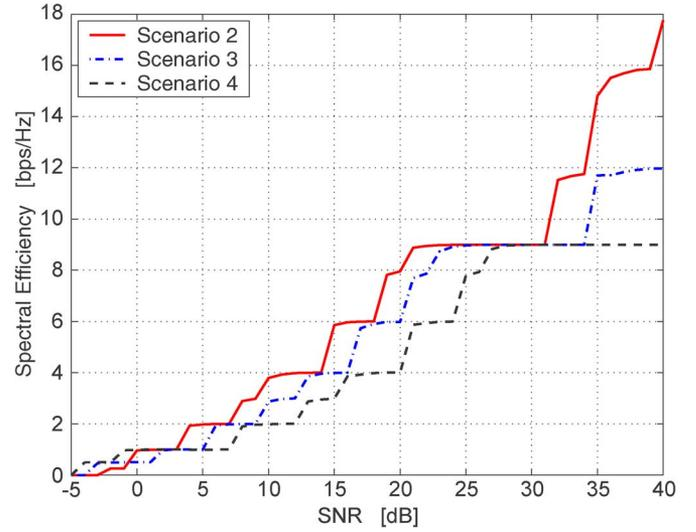
Fig. 8. Spectral efficiency of the adaptive MIMO transmission scheme in different channel scenarios.
