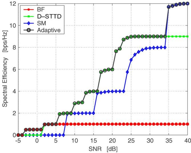
Fig. 7. Spectral efficiency of the adaptive MIMO transmission scheme versus fixed BF, D-STTD, and SM with adaptive MCS, in channel scenario 3 in [10].
