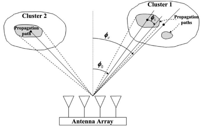
Fig. 1. Geometry of the model representing clusters and propagation paths. The angles  $\phi_c$  and  $\phi_0$  are the mean AOAs of the cluster and propagation paths, respectively. The angle  $\phi_i$  is the AOA offset of the path.
