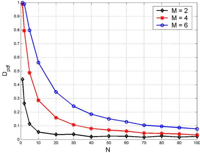
Fig. 4. Distance between the pdf of  $C$  as a function of the number of rays for PM and ENPM. The same number of transmit/receive antennas (i.e.,  $M_t = M_r = M$ ) and single cluster channel with AS  $\sigma_\phi = 50^\circ$  and  $\phi_0 = 0^\circ$  was used.
