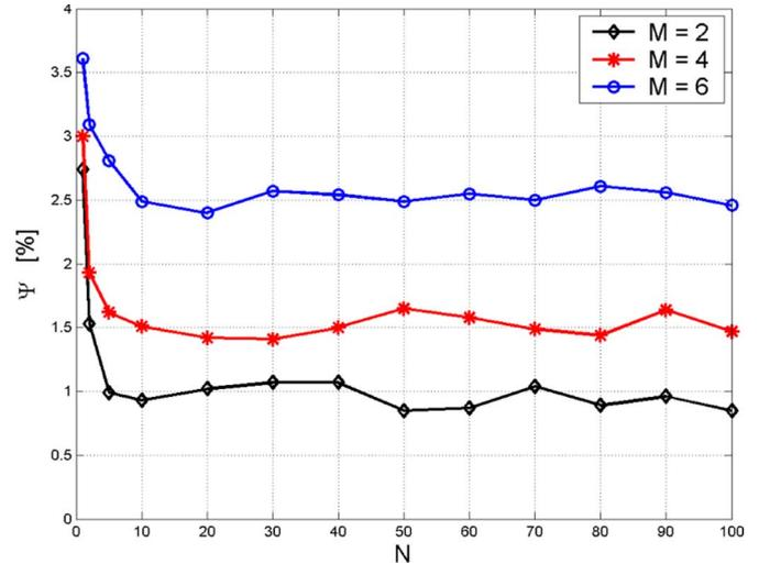
Fig. 5. Distance  $\Psi$  between the spatial correlation matrices for PM and ENPM. ULA is assumed with  $M_t = 4$ ,  $M_r = 1$ . The channel is simulated with  $\phi_0 = 0^\circ$  and different values of  $\sigma_\phi$ .
