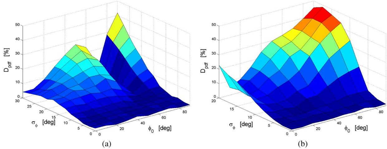
Fig. 6. Distance between the pdf of  $\Omega$  as a function of AS and mean AOA for PM and ANPM. The same number of transmit/receive antennas (i.e.,  $M_t = M_r = M = 4$ ) is assumed with ULA and UCA. (a) ULA. (b) UCA.
