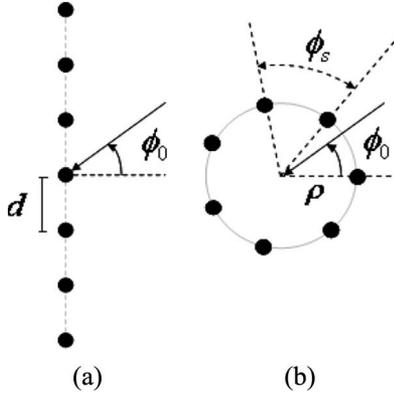
Fig. 2. ULA and UCA configurations, seven-element case. (a) ULA. (b) UCA.
