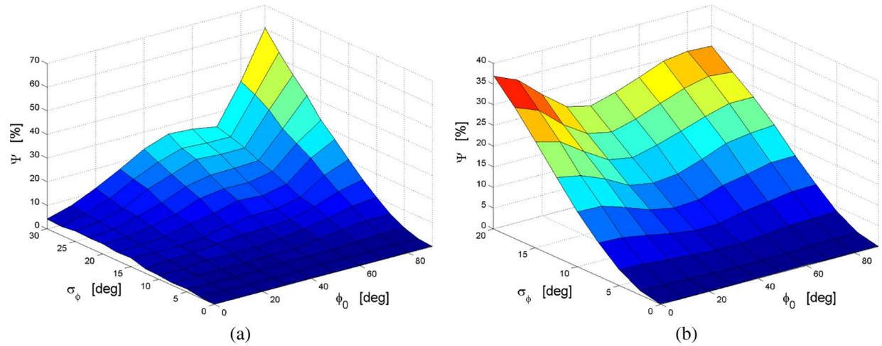
Fig. 7. Distance  $\Psi$  between the spatial correlation matrices for PM and ANPM. The same number of transmit/receive antennas (i.e.,  $M_t = M_r = M = 4$ ) with ULA and UCA. (a) ULA. (b) UCA.
