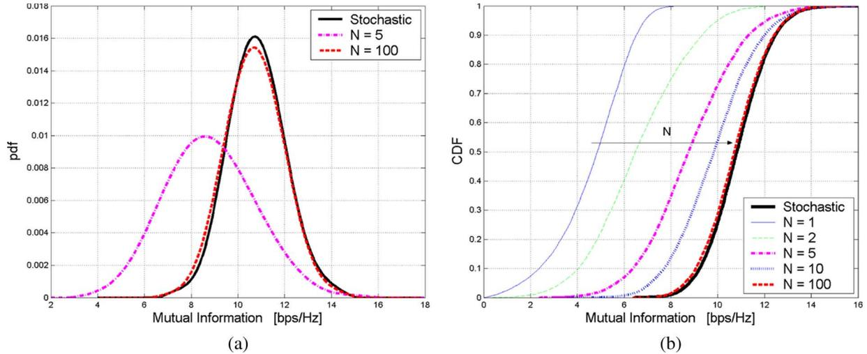
Fig. 3. PDF and CDF of the mutual information for PM and ENPM with variable number of rays ( $N$ ). The same number of transmit/receive antennas (i.e.,  $M_t = M_r = 4$ ) and single cluster channel with  $\sigma_\phi = 50^\circ$  and  $\phi_0 = 0^\circ$  was used. (a) PDF. (b) CDF.
