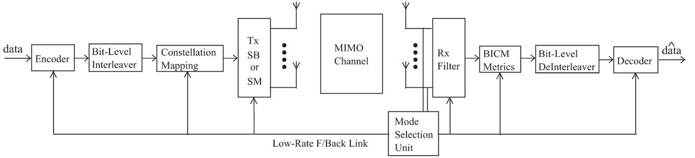
Fig. 1. MIMO BICM system architecture.
